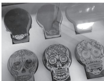
Skulls in the process of being laser engraved.
